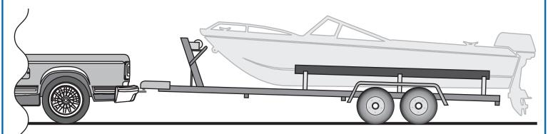
Trailer is not level, note that most of the load is on the rear axle
