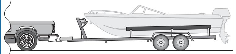
Trailer is not level, note that most of the load is on the front axle
