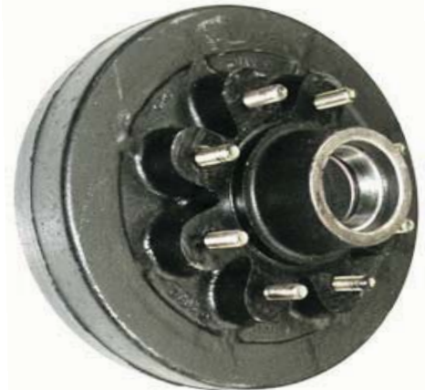
8 Lug hub Drum with 1 3/4" inner brg # 25580 & 1 1/4" outer brg
