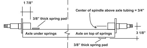
Axle drop for 2 x 2 axle with axle under the springs=
