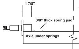
Center of spindle above axle tubing = 3/4"
